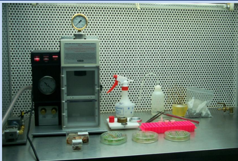
Fig. 2. Gene gun used for genetic transformation in potato
