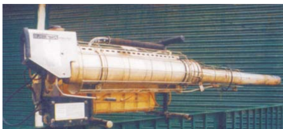
Fig. 8. A fogging machine (Dyna fog, USA) used for CIPC application
