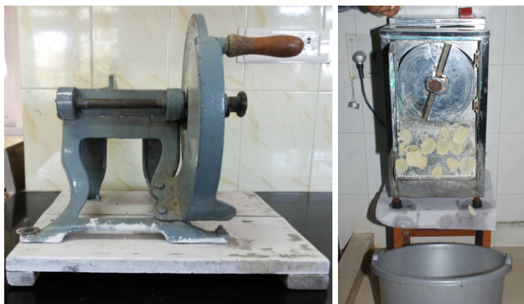
Figure 25: Manual and electrical potato slicer for making chips
