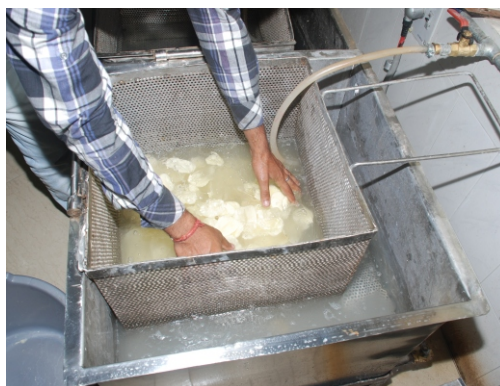
Figure 27: Blanching of potato slices for making chips
