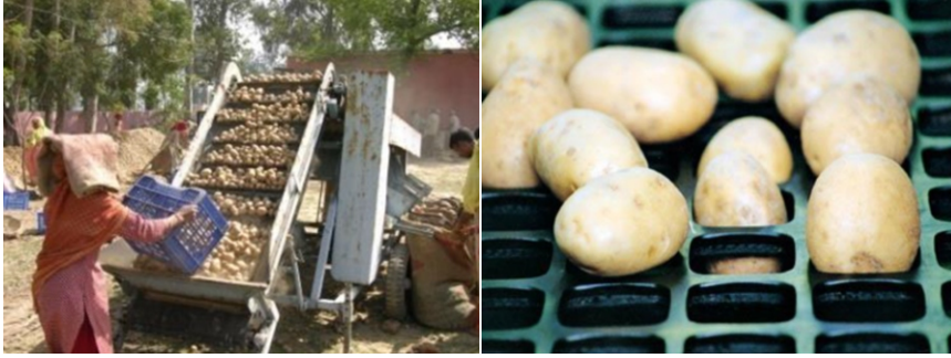
Figure 23: Mechanical grading of potatoes
