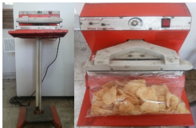
Figure 31: Small scale packaging machine and packed potato chips
