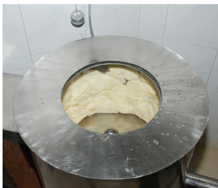
Figure 28: Spin dryer with potato chips
