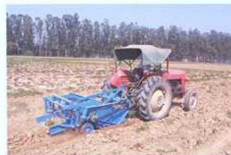
Potato digger shaker for stage II
