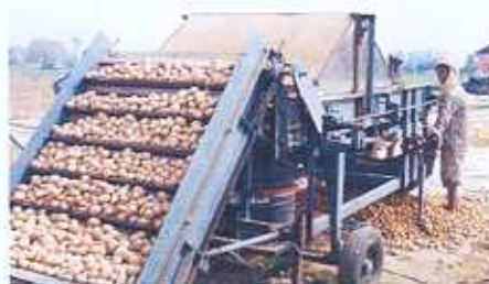
Fig. 11 Potato seed tuber treatment with boric acid through seed treatment device
