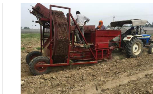
Fig. 3. Two row Potato combine harvester
