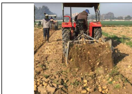
Fig. 1. Tractor operated digger elevator
