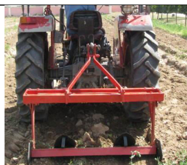
Fig. 2. Low cost blade type digger
