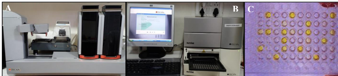
Fig. 2. Automated ELISA facility with robotic plates washer (A), plate reader (B) and visual observation ELISA plate with yellow coloured wells indicating positive for virus (C).
