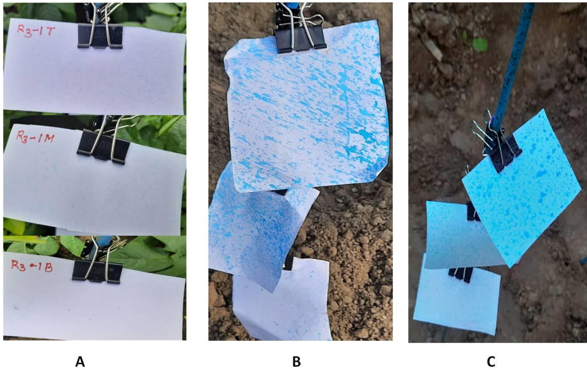
Fig.3. Droplet distribution (A) Drone spray; (B) Tractor mounted spray; (C) Battery operated knapsack spray
